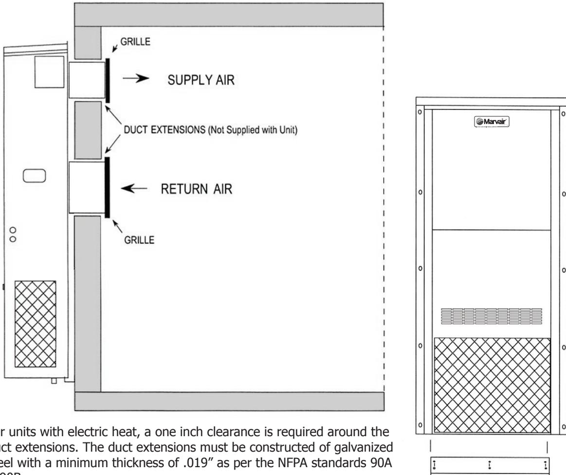
For units with electric heat, a one inch clearance is required around the duct extensions. The duct extensions must be constructed of galvanized steel with a minimum thickness of .019" as per the NFPA standards 90A & 90B.
