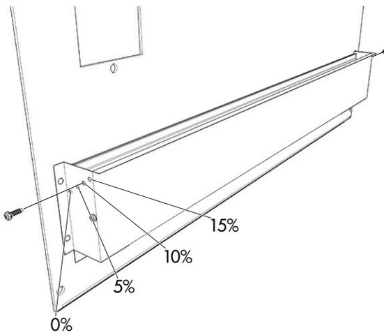
**Figure 3a. Fresh Air Hood Damper for AVPA20-60**
