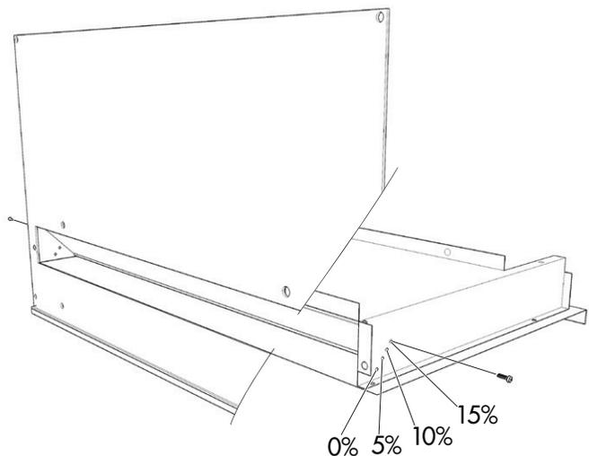
**Figure 3b. Fresh Air Hood Damper for AVPA12**
