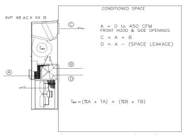
**Figure 2. Damper Air Path**
