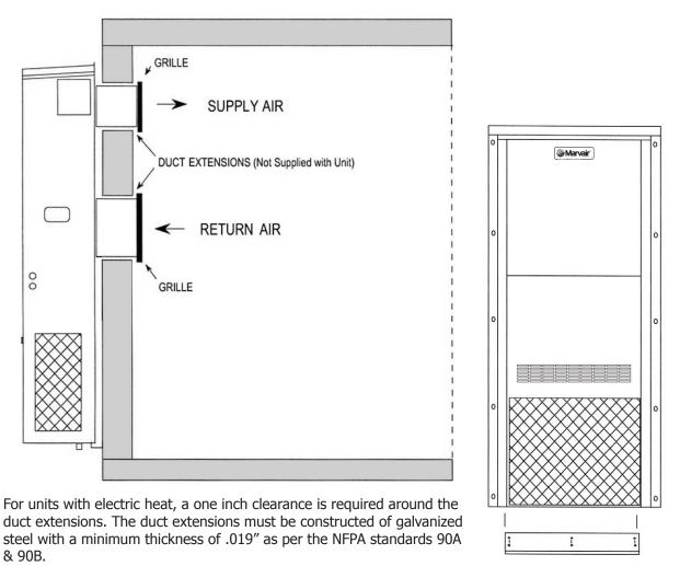
Figure 4. Wall Mounting Detail - Models AVPA12-60
