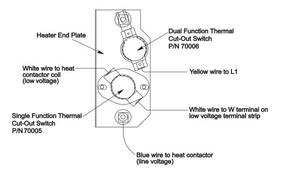
**Figure 6. Typical Configuration for Single Element Heater**
