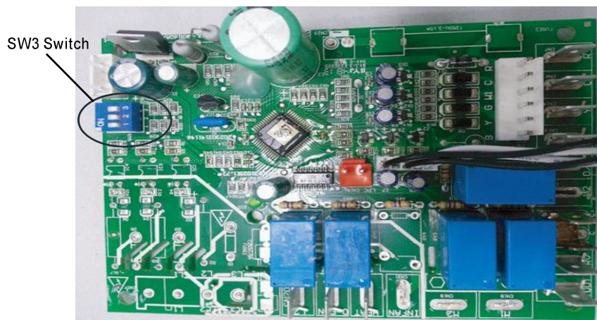
Fig.11 SW3 Switch Location in the PCB Board
