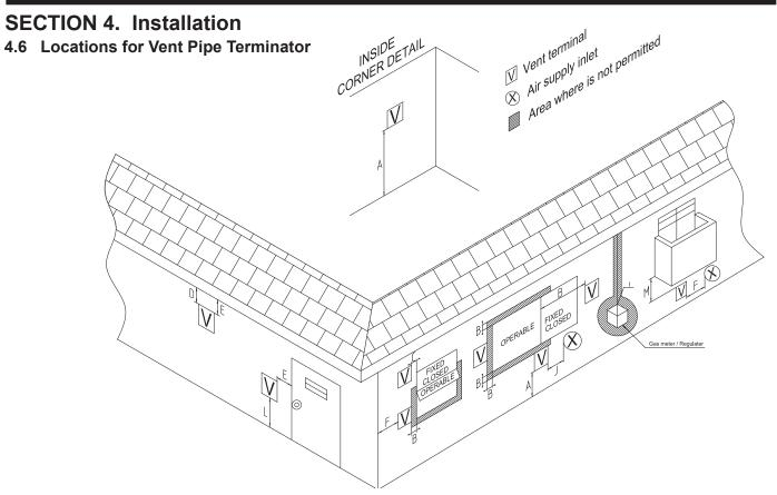
\* For clearances not specified in ANSI Z224.1 / NFPA 54 or CAN/CSA-B 149.1, please use clearances in accordance with local installation codes and the requirement of the gas supplier.
