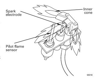
Figure 22 Typical main burner flame
