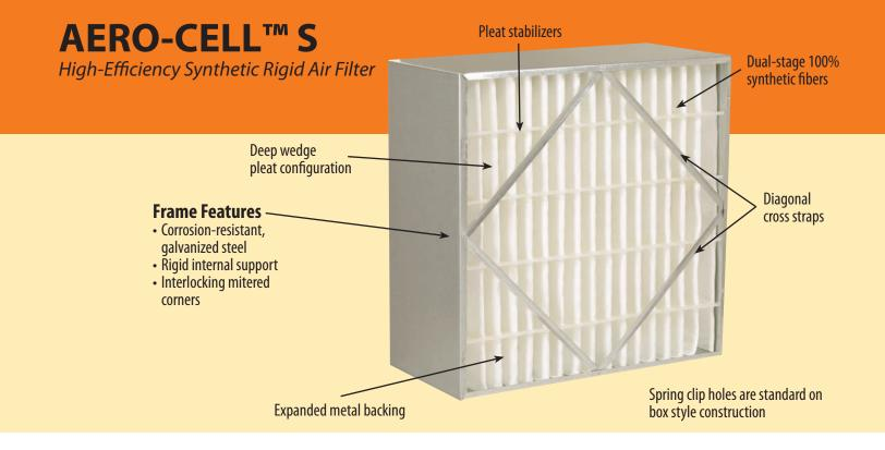
In an effort to respond to the increasing synthetic media requirements of the air filtration industry, Purolator offers the AERO-CELL<sup>TM</sup> S rigid box filter, a rigid air filter engineered to provide medium and high-efficiency filtration combined with a prolonged life cycle. Its box filter construction eliminates the need for retainers and special external wire media supports.
