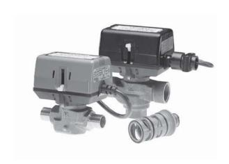
These 2-position (open/close) control actuators are used with VCZ1000, 1100, 6000 and 6100 series hydronic valves in a normal indoor environment to provide quick opening/closing to control the flow of hot and/or chilled water or glycol solution to 60% concentration. They are designed for on-off "zone" control of heating/cooling systems, or to control individual fan coil, baseboard radiator or convector applications.
