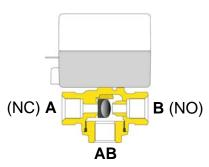
**3-way valve with normally closed actuator** (Note: 3-way uses only normally closed actuator)
