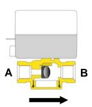
2-way valve with normally closed actuator
