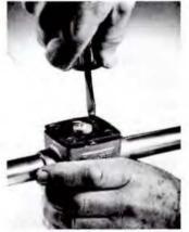
2-Remove the 4 Screws from hold down plate
