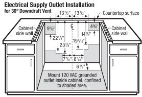
Electrical Installation Notes: All vertical dimensions relative to top surface of countertop; all horizontal dimensions relative to cutout in countertop. Locate grounded electrical outlet for 28"-long power cord within reachable distance. When installing vent in 30"-wide cabinet, outlet cannot be located on back wall of cabinet, but can be wall-mounted with access hole in cabinet, Ensure that access to outlet will NOT be obstructed by ducting after installation.
