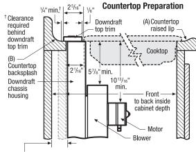
Maximum 41/2" gap allowed between inside cabinet back and chassis BEFORE downdraft stabilizing brackets will require wood support installation for mounting
