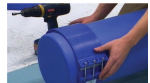
Slide clamp over gasket and tighten screws
