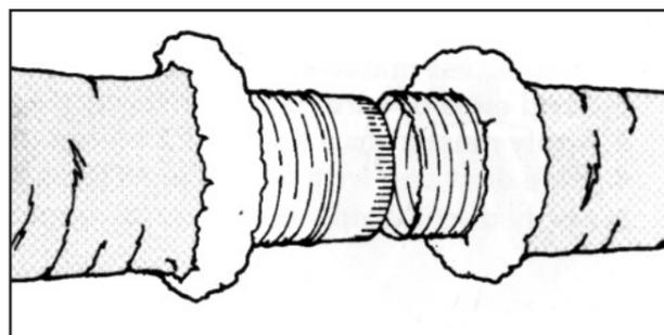
2. Tape cores together with at least 2 wraps of duct tape. Secure connection with 2 clamps placed over the taped core ends and past the beads.
