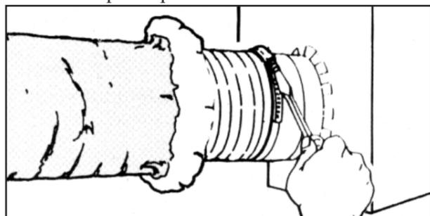
3. Pull jacket and insulation back over core. Tape jacket with at least 2 wraps of duct tape. A clamp may be used in place of or in combination with the duct tape.
