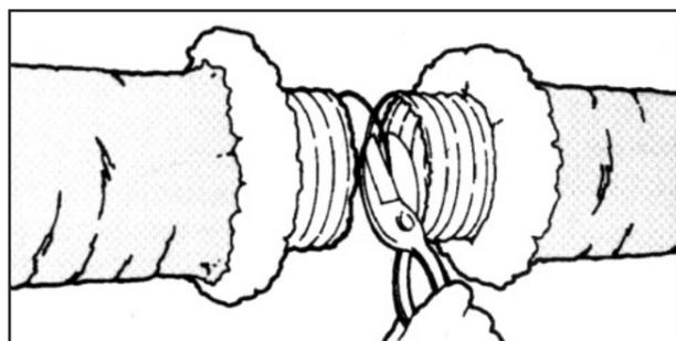
2. Slide at least 1" [25 mm] of core over fitting and past the bead. Seal core to collar with at least 2 wraps of duct tape. Secure connection with clamp placed over the core and tape and past the bead.
