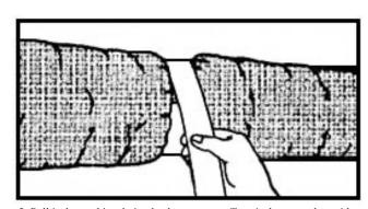
3. Pull jacket and insulation back over cores. Tape jackets together with at least 2 wraps of duct tape. A clamp may be used in place of or in combination with the duct tape.
