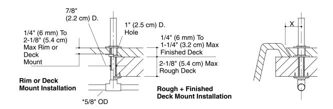
\* Indicates items to be supplied by installer. X= Distance from centerline of spout inlet to front of spout base plus 1/2" (1.3 cm).
