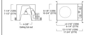
Cut-out: 4-3/8" ID: 4" Housing Length: 12-11/16" (120V) 17-3/4" (277V) Housing Width: 8-1/8" (120V) 10-3/4" (277V)
