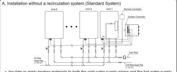
• Insulate or apply heating materials to both the cold water supply piping and the hot water supply piping to prevent freezing during cold weather and to prevent heat loss through the piping.
