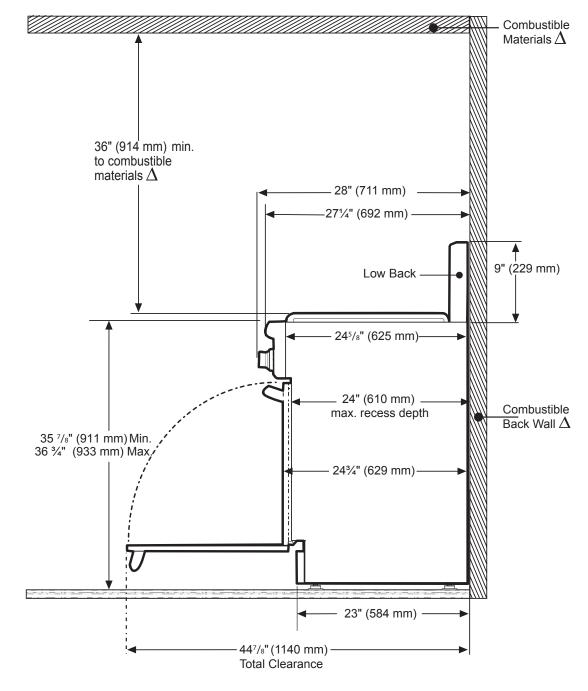
$\Delta$  As defined in the "National Fuel Gas Code" (ANSI Z223.1, Current Edition). Clearances from non-combustible materials are not part of the ANSI Z21.1 scope and are not certified by CSA. Clearances of less than 12" (305 mm) must be approved by the local codes and/or by the local authority having jurisdiction.
