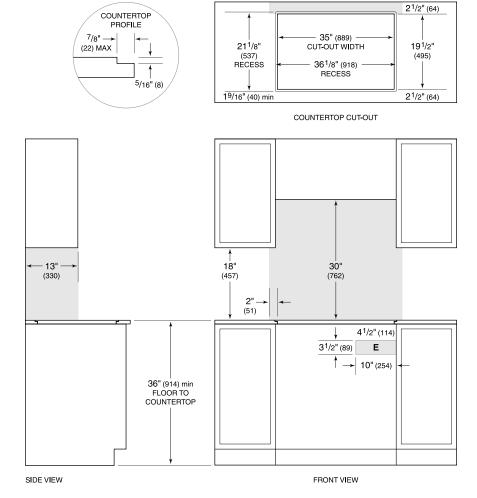
NOTE: Shaded area above countertop indicates minimum clearance to combustible surfaces, combustible materials cannot be located within this area. Electrical supply location only applies to installations with built-in oven. Outside comer radius 7/16" (11).
