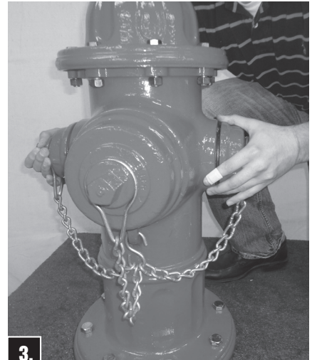
3. Rotate Upper Barrel section as desired.
