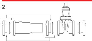
Disassemble the gland and gasket from the sleeve and interchange with the gland and gasket from one end of the cut-in valve.
