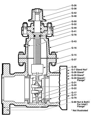
\*\* Cast iron discs with rolled-in bronze facings; cast iron top wedge nut with integrally cast bronze busing.
