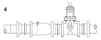
Position cut-in valve on end of main. Slide sleeve spigot end into end of valve. Tighten stop screw so it clears end of pipe.
