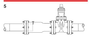
Position gaskets and glands. Install all tee-head pipe gland bolts and tighten. Open the cut-in valve and turn on water pressure in main.
