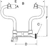
P-1479-6DN for the ASSE approved top entry vertical check with a test drain;
