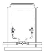
M.I.P. meter thread ends - used to retrofit dual check with sampling to existing meter set (203H1445----02N shown)
