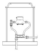
Integral Mueller Pack Joint vertical inlet for CTS O.D. tubing and horizontal outlet with multi-purpose connection (P-1476N shown) Typical installation of a vertical inlet and horizontal outlet copper meter yoke
