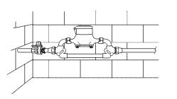
Multi-purpose thread ends (H-2518-2N shown) Typical installation of a straight line inlet and outlet copper meter yoke
