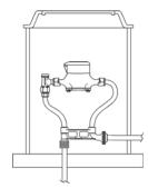
MIP vertical inlet and horizontal outlet with multi-purpose connection (H-1568N shown)
