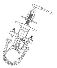
The drilling and tapping tool is extracted and a corporation stop is attached to the boring bar for insertion into the main.
