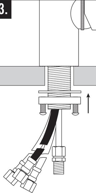
Slide washer and thread the clamp nut onto threaded shroud. Tighten nut snug to underside of sink or counter.
