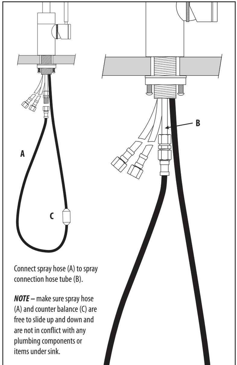
Connect spray hose (A) to spray connection hose tube (B).
