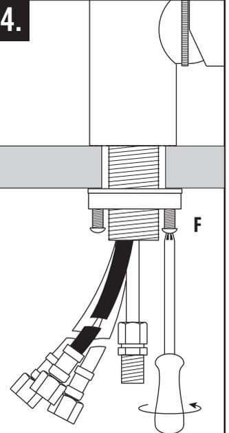
Turn faucet to the desired handle position. Securely tighten clamp screws (F).
