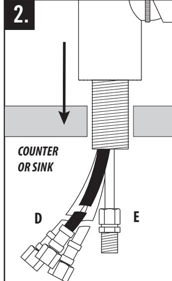
Fit flexible hoses (D) and spray connection tube (E) through hole on counter or sink. *(No plumbers putty is required. O-ring seals base).*
