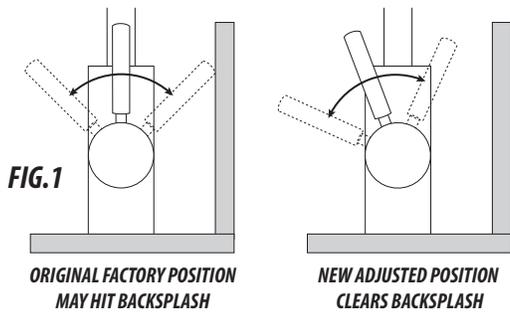
On some kitchen countertops, the handle may hit the backsplash when the faucet handle is positioned to the left or right (Fig. 1). Waterstone gives you the option of adjusting the handle 22.5 degrees to avoid hitting backsplash.
