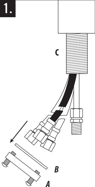
Remove the clamp nut (A) and washer (B) from the threaded shroud (C).
