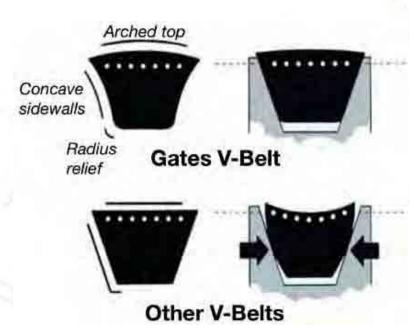
When V-belts are under tension and running in a sheave they change shape. To optimize power transmission, many Gates V-belts are designed with the exclusive Gates Curves feature. Gates Curves consist of three key components: concave sidewalls, radius relief corners and an arched top.
