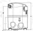
Notes Large CRKQ Mounting pattern 7.5\*x 7.5\* Length 10,62\* by width 9,23\* Suction diameter 7/8" elbow up Add 0.28" to height if grommets included Discharge height is 6.24"
