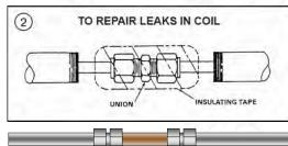
These kits are to be used for repair of aluminum coils only. Use on copper coils can cause leaks even though properly Installed.
