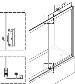
**19** With help, lift the outside panel onto the track and over the guide. Ensure the rollers operate smoothly. Refer to the Troubleshooting table as needed.
