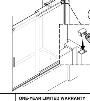
**29** Apply 100% silicone sealant along the wall jambs inside and outside the shower, and apply along the threshold outside the shower.
