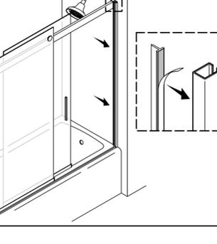
**28** Apply a small bead of 100% silicone sealant to the underside of the wall jamb cap. Press the cap onto the wall jamb.
