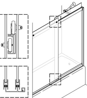
**20 Important!** Position the screws at the dimensions shown. Drill 5/32" holes into the retainer. Slide the retainer between the panels. Secure to the header with six screws.
