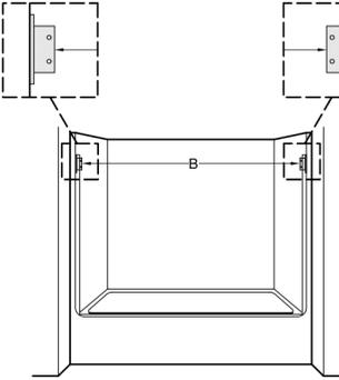
**14 Important!** Do not cut the header too short. Add 1" (25 mm) to "B" and cut the header and retainer.
