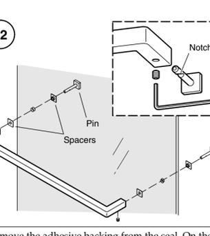
**23 Handle models:** mark distance "C" on the glass. Use alcohol wipes to clean the glass at the handle installation location. Ensure the inside panel is closest to the showerhead.
