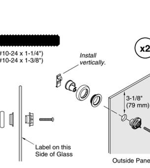
**18** With help, lift the inside panel over the guide and into the track. Ensure the rollers operate smoothly. Refer to the Troubleshooting table as needed.
