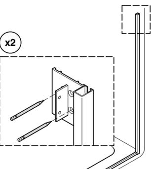
**11** Drill 5/16" holes at the two diagonal cleat marks. Insert anchors.
