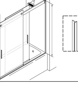
**27** Remove the adhesive backing from the seal. On the side closest to the showerhead, attach the seal to the shower side of the wall jamb.
