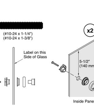
**17 Outside panel:** install an outside roller, clip, and screw in each upper hole. Ensure the clip is vertical.
