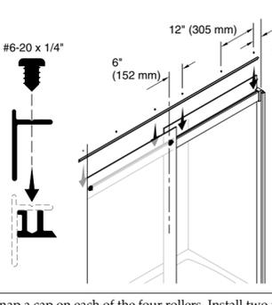
**21** Apply 100% silicone sealant to the back of the bumper. Open the bumper and install over the cleat. Press tight to engage the tabs.
