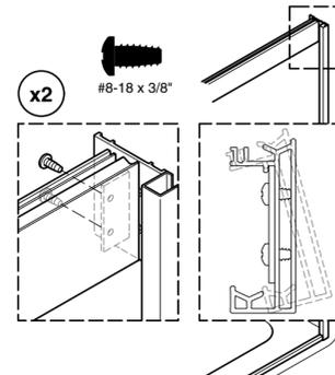
**16 Inside panel:** install the inside rollers and screws in the upper holes.
