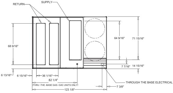
Figure 4. Gas/electric units — plan view — 15–25 tons standard efficiency
