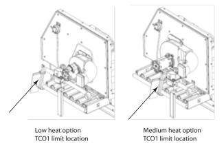
3. Replace and discard the existing TCO1 originally installed at the factory for down flow operation with the TCO1 from Step 2 for horizontal operation.
