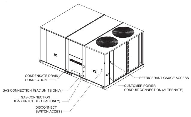
Figure 3. Gas/electric units — front & side views — 15–25 tons standard efficiency
