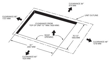
Figure 8. Downflow unit clearance — 15–25 tons standard efficiency
