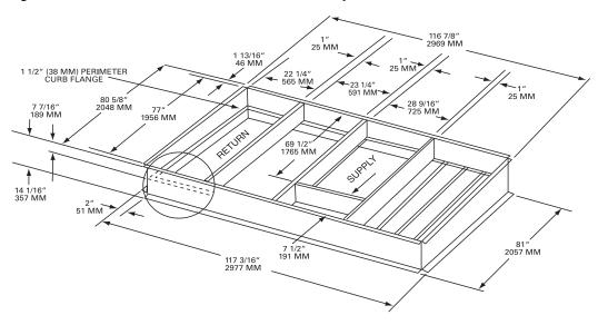
Figure 7. Downflow duct connections—field fabricated 15-25 tons standard efficiency
