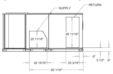
Figure 6. Roof curb - 15-25 tons standard efficiency
