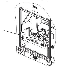
3. Install the vent hood on the gas heat panel using the screws removed in Step 1. Make sure it is properly secured on to the panel.
