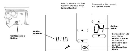
Note: Configuration mode automatically ends if no buttons are pressed for 10 minutes.
