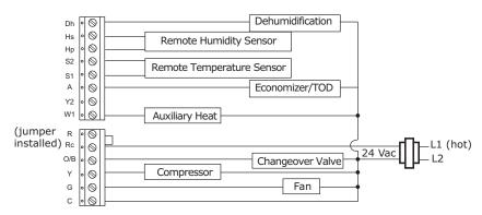
Figure 10. Programmable Thermostat, 2H/2C, Conventional (Option 7)
