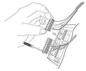
3. Push the excess wire through the hole in the wall cavity or into the junction box.
