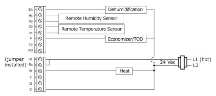
Figure 7. Programmable Thermostat, 1H, Conventional With Fan (Option 4)
