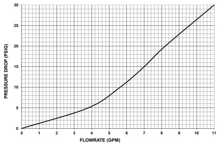
Cold and hot water inlet pressures at 45 psig; Cold water supply temperature at 55  $\pm$ 5 °F; Hot water supply temperature at 140  $\pm$ 5 °F; Mixed water temperature at 105  $\pm$ 5 °F.
