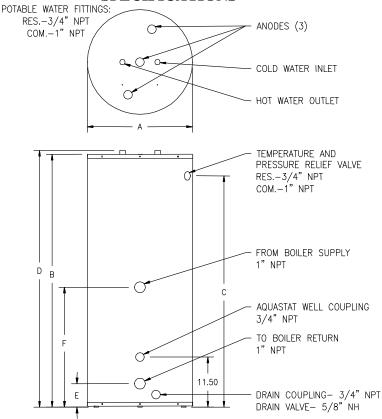
Figure 1 - Tank Layout
