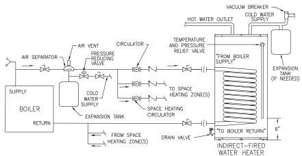
Figure 3 - Water Boiler Piping with Circulators
