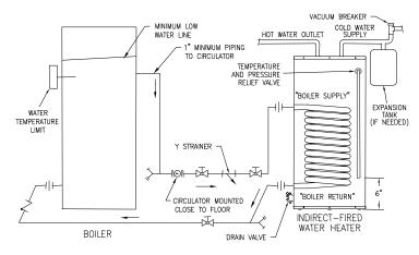
Figure 4 - Typical Steam Boiler Connections (connections available below the water line)
