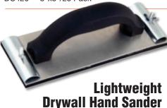
Lightweight aluminum back. Available with wood or plastic handle. Clamps lock sandpaper tight to base. Sander face is 9-1/2"x3-1/4".
