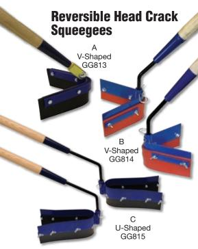
Reversible head allows a push or pull action to funnel material into cracks. Choose between V or U-shaped black Neoprene blade that withstands temperatures up to 220°F. V-shaped red silicone blade withstands temperatures up to 450°F. Each includes a 54" heavy-duty wood handle. Blades are reversible.
