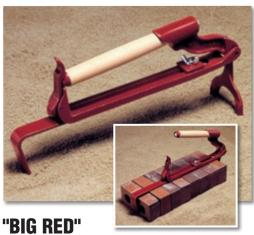
Non-slip lock down to unload quickly and easily. Will not damage bricks and is designed and built for long wear. Large wing nut makes for fast adjustment from 7 to 11 bricks. Made of malleable iron with smooth wood handle. A favorite with brick masons across the country.
