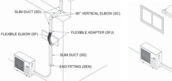
WALL INLET (SW) 90° FLAT ELBOW (SK) - SLIM JOINT COUPLER (SJ) - SLIM DUCT (SD) END FITTING (SEN) A precision engineered system of prefabricated PVC ducts which are designed to conceal and protect external surface mounted refrigeration line sets. They can also be used to conceal drain hoses and electrical wiring. SlimDuct is weather resistant and available in three colors: ivory, white, or brown. Installation is simple with easy access for the technician.
