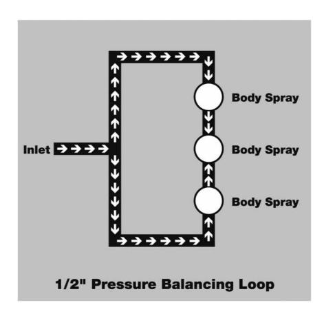
Note: Pressure-Balance Loop should be used on each shower bar installed.
