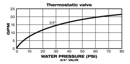
3) Exceeding the capacity of the valve will result in the reduction of the overall performance of the shower. Since water pressure directly facilitates optimum performance, Newport Brass recommends a minimum of 50 pounds per square inch (psi) for 3 or more outlets.
