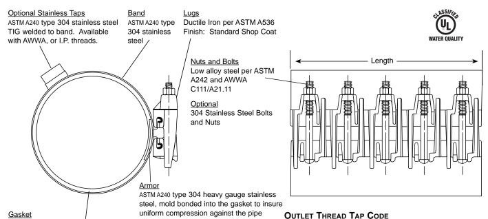
Gridded Virgin SBR compounded for water service, per ASTM D2000. Buna-N, Nitrile, is available as optional material.
