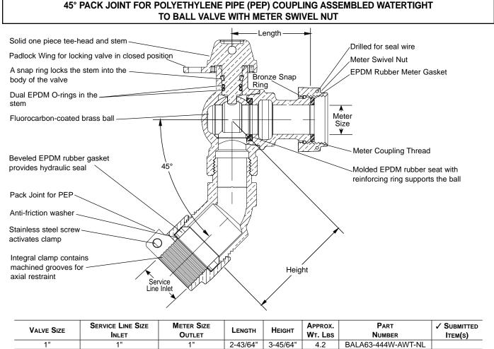
Note: Ford recommends using insert stiffeners with plastic pipe or tubing.
