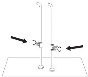
8. Apply thread sealant to the inlets on the back of the faucet body. Attach the faucet to the upper riser pipes and tighten the slips nuts to secure.
