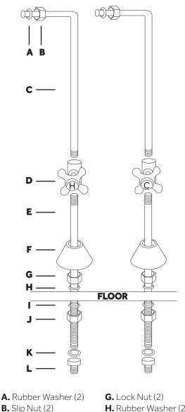
**C.** Upper Riser Pipe (2) **D.** Straight Stop Valve (2) **J.** Lock Nut (2) **E.** Lower Riser Pipe (2)
