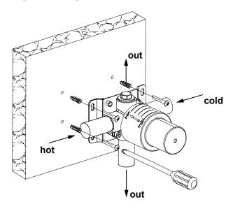
Install the valve body. Wrap the threaded portion of the joints in Teflon tape and connect the water inlet and outlet.
