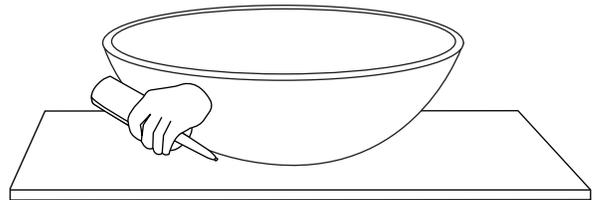
4. Remove any excess sealant with a damp cloth to complete installation.
