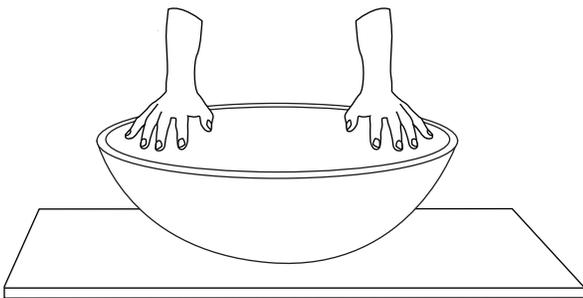
3. If desired, apply a continuous bead of silicone sealant around the perimeter of the sink base for additional stability.
