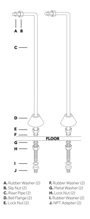
1. Slide the slip nuts (B) up the upper riser pipes (C).
