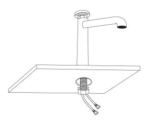
3. From beneath the sink, slide the rubber washer back onto the faucet body. Thread the locknut back onto the shank until hand tight. Finish tightening using a basin wrench.
