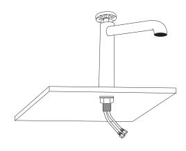
4. Apply plumber's tape or thread sealant to the threading on each of the faucet's water lines, and connect the main water hoses to the faucet. Use an adjustable wrench to tighten, but be careful not to overtighten. Ensure that you are connecting the hot and cold lines appropriately.
