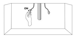
6. Proceed to the drain installation. Once complete, remove the aerator from the spout and turn the faucet on for approximately 60 seconds to remove any dust or loose sediment from the water lines. Ensure that there are no leaks, and that both hot and cold water are running properly. Turn the water off and reattach the aerator.
