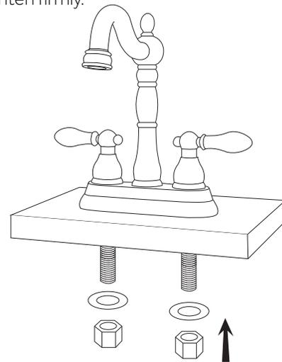
4. Connect the main water supply lines to the threaded shanks of the faucet. If necessary, use the provided brass nuts and cone washers to make the connections. Use an adjustable wrench to tighten, but be careful not to overtighten. Apply thread sealant or plumber's tape to the threads before attaching.
