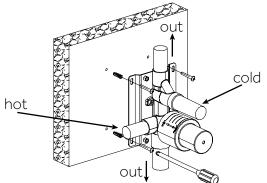
1. Install the valve body. Wrap the threaded portion of the joints in Teflon tape and connect the water inlet and outlet.
