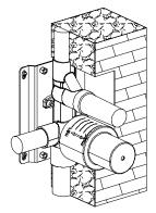
2. Put the protective covers on the valve body and finish the shower wall.
