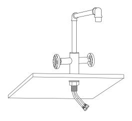
4. Apply plumber's tape or thread sealant to the threading on each of the faucet's water lines, and connect the main water hoses to the faucet. Use an adjustable wrench to tighten, but be careful not to overtighten. Ensure that you are connecting the hot and cold lines appropriately.
