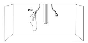
6. Proceed to the drain installation. Once complete, remove the aerator from the spout and turn the faucet on for approximately 60 seconds to remove any dust or loose sediment from the water lines. Ensure that there are no leaks, and that both hot and cold water are running properly. Turn the water off and reattach the aerator.
