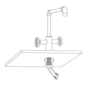
3. From beneath the sink, slide the rubber washer back onto the faucet body. Thread the locknut back onto the shank until hand tight. Finish tightening using a basin wrench.
