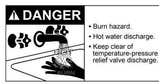
It is recommended that the temperature-pressure relief valve be checked to ensure it is in operating condition at least once a year.
