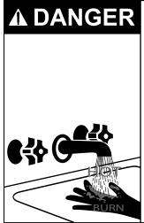
Water temperature over 125°F can cause severe burns instantly resulting in severe injury or death.
