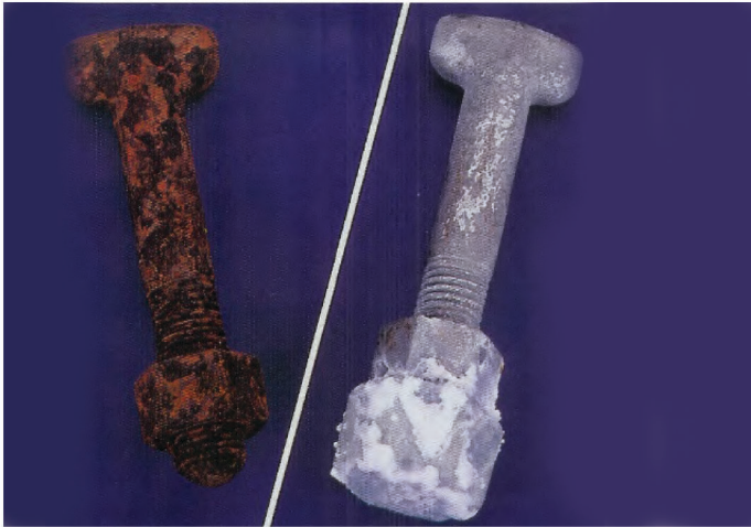
Submerged in concentrated salt water for 5,000 hours.
