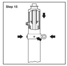
**Step 15.** Engage Extension Rod by Operating Stem and install Cap Assembly on Post Assembly. Install and tighten Screw, Washer, and Eyebolt. Tighten Set Screws to secure.
