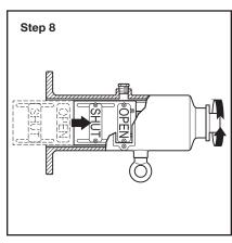
**Step 8.** Position Target Carrier in Cap cavity and engage Operating Stem by Stem Nut. Rotate Operating Stem clockwise until OPEN Targets are centered in Cap windows.
