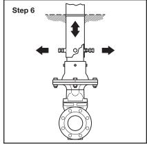
**Step 6.** Loosen Screws and Lock Nuts securing Upper Pipe to Lower Pipe. Adjust Upper Pipe, aligning Mark Ring height with finished grade.
