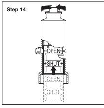
**Step 14.** Position Target Carrier in Cap cavity and engage Operating Stem by Stem Nut. Rotate Operating Stem clockwise until OPEN Targets are centered in Cap windows.
