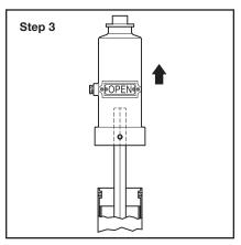
**Step 3.** Remove Cap Assembly from Post Assembly.
