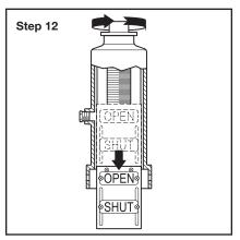
**Step 12.** Rotate Operating Stem counterclockwise to remove Target Carrier from Cap.
