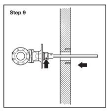
**Step 9.** Install Extension Rod Assembly engaging Gate Valve Top Cap by Connect Cap. Tighten Connect Cap Set Screws to secure.
