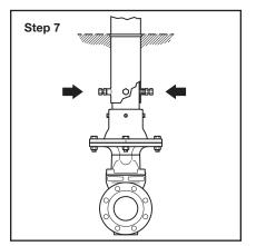
**Step 7.** Tighten Screws and Lock Nuts to secure Upper Pipe to Lower Pipe.
