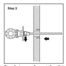
**Step 3.** Loosen Connect Cap Set Screws. Insert Extension Rod Assembly through wall clearance hole and temporarily engage Gate Valve Top Cap by Connect Cap.
