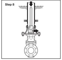
**Step 8.** Loosen Connect Cap Set Screws. Temporarily Install Extension Rod Assembly in Post Assembly, engaging Gate Valve Top Cap by Connect Cap.
