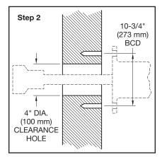
**Step 2.** Cut hole in wall for Connect Cap clearance. Drill four anchor bolt holes on 10-3/4 inch (273 mm) BCD for securing Post Body to wall in orientation shown in Step 10.
