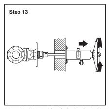
**Step 13.** Rotate Handwheel clockwise until OPEN Targets are centered in Cap windows. Ensure that Gate Valve is fully open.
