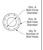
FIGURE 2 GATE VALVE FLANGE NOMINAL DIMENSIONS
