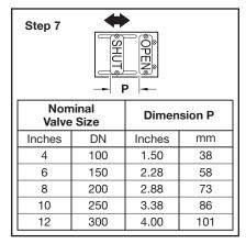
**Step 7.** Loosen SHUT Target Screws and Nuts and adjust position per table above. Tighten Screws and Nuts. Repeat for opposite side of Target Carrier assembly.
