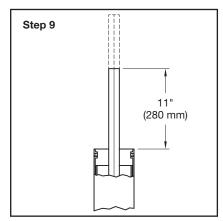
**Step 9.** Mark Extension Rod 11 inches (280 mm) above top of Upper Pipe. Remove Extension Rod Assembly. Evenly cut Extension Rod at marked location.
