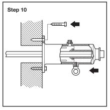
**Step 10.** Engage Extension Rod by Operating Stem and guide Cap Assembly into position over anchor bolt holes. Hold in place and secure with four anchor bolts (not included).
