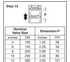
**Step 13.** Loosen SHUT Target Screws and Nuts and adjust position per table above. Tighten Screws and Nuts. Repeat for opposite side of Target Carrier assembly.
