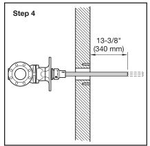
**Step 4.** Mark Extension Rod 13-3/8 inches (340 mm) from wall. Remove Extension Rod Assembly and evenly cut extension Rod at marked location.
