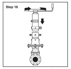
**Step 16.** Engage Operating Stem with Wrench. Rotate Wrench counterclockwise until SHUT Targets are centered in Cap windows. Ensure that Gate Valve is fully shut.
