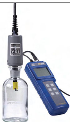
DO200 instrument with laboratory BOD probe (200-BOD).
