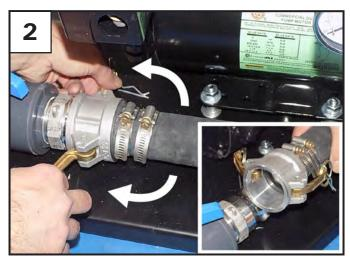
Loosen clamps on cam fitting & disconnect hose.
