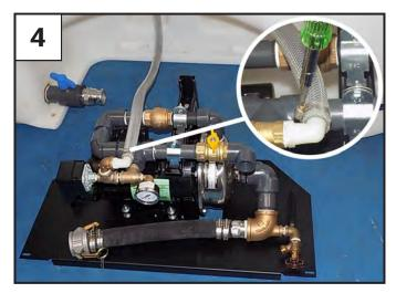
Continue to pull the pump assembly out by the base plate handles & disconnect the test hose.
