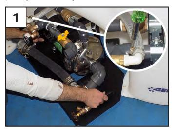
Using the handles on base, slide the left side of pump assembly into the tank opening & connect test hose.
