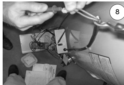
8 Checking continuity of upper sensor wire harness.
