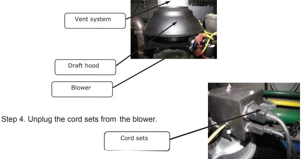
Step 5. Remove the (3) blower mounting screws using a 1/4" nut driver and retain for later use.
