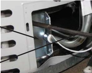
Step 6. Remove the connectors attached to the resettable thermal switch on the right side inner door.
