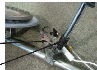
Step 10. Visually inspect the spark igniter/flame sense wire for damage. Replace the pilot assembly, if damage is found.
